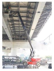
Apart from being highly durable and able to boost productivity, these AWP machines are equipped with IIIA engines to reduce noise during use to as low as 106 decibels.
